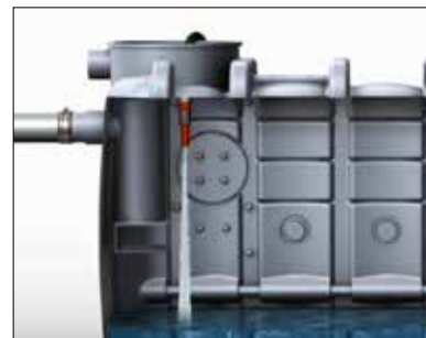
Example: Filling of separator via open cover and water hose
